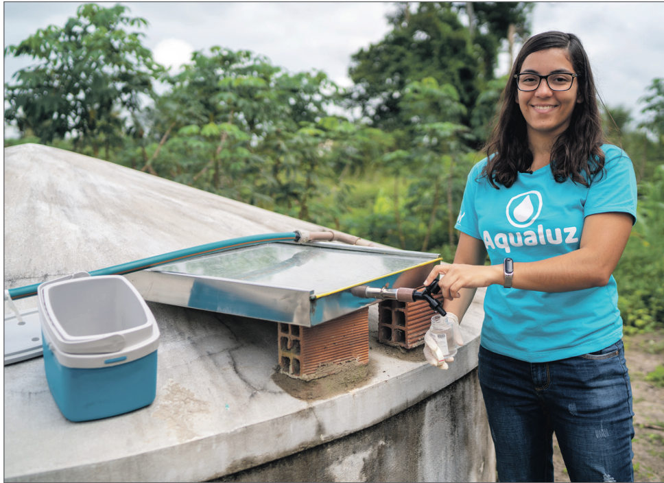
Anna-Luisa Beserra getting clean water from the Aqualuz. The Aqualuz is mounted on a concrete cistern that stores rainwater.
