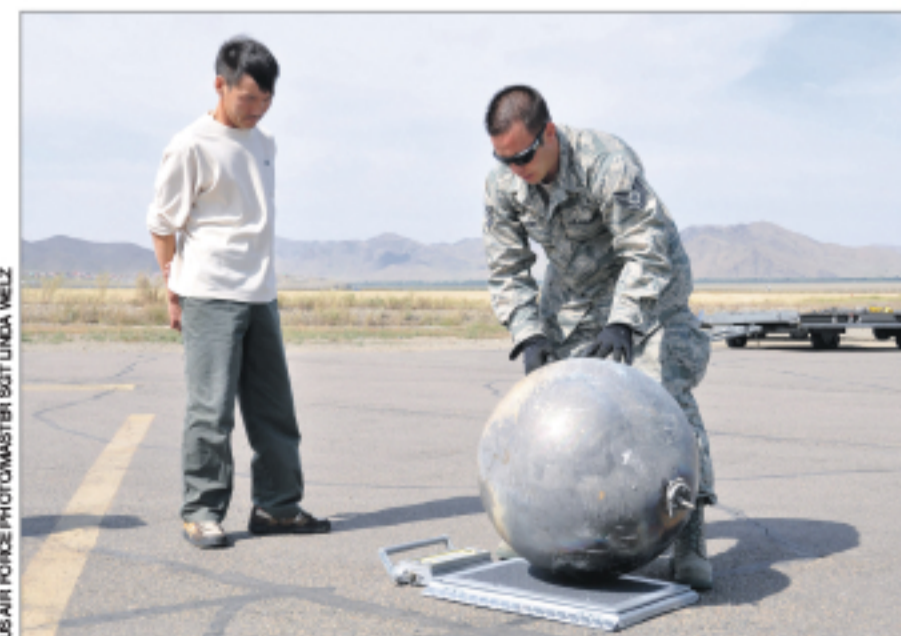
Technical Sergeant John Lowe (right) weighs a hydrogen fuel tank, part of the debris from a Delta II rocket launch in 2010. The crew returned the debris to the Space and Missiles Systems Center at Los Angeles Air Base in California.
