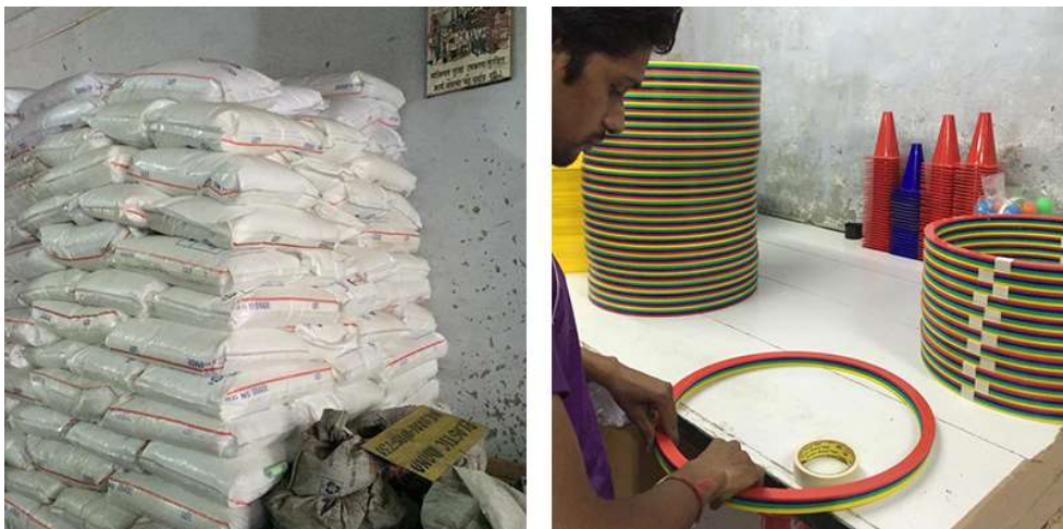
In India: Plastic pellets arrive in a factory in India in 100kg sacks (left). The pellets will be melted and moulded to form hula hoops. These are packed by workers (right) for transport by road and ship. [Photos: Jeremy Ko]
