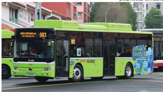
Yutong E12, SMRT Buses, since 2020 Features: 80 passengers; Fully electric Emissions standards: Zero emissions
