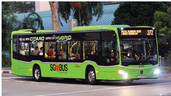
Mercedes-Benz Citaro Hybrid, SBS, since 2020 Features: 93 passengers; Diesel and electric hybrid Emissions standards: Euro 6
