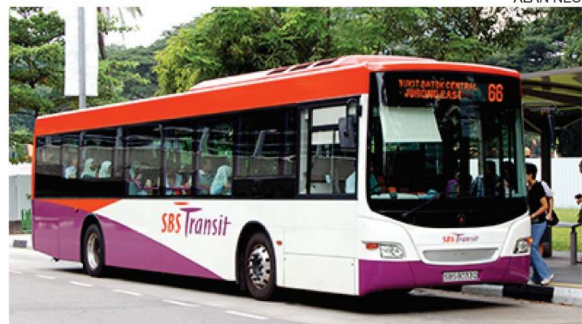
Scania K230UB, SBS Transit, since 2007 Features: 87 passengers; Wheelchair accessible, low entry. Emissions standards: Euro 4
